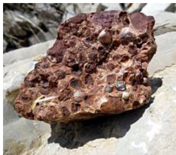
Figura 8.11. Bauxita, mena de aluminio. By Isidre blanc (Own work) [CC BY-SA 3.0], via Wikimedia Commons.
